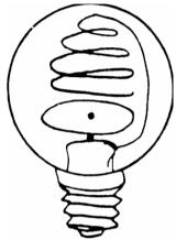
Fig. 7: 'Osglim' type of neon glow lamp
